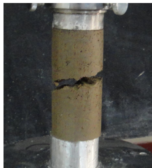
图 3 土样破坏的照片 Fig.3 Photo of failure of soil sample
